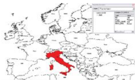
Fig. 1. Vector map of Europe and attribute (spreadsheet), used in this example to extract Italy.
